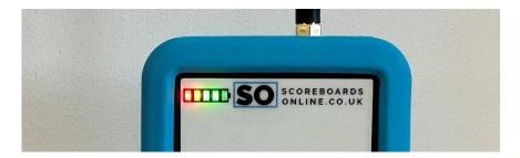
To fully charge the controller, it can take up to 8 hours. If necessary, the remote can be used whilst it is charging. When charging, the red light underneath the soft cover will be lit. When fully charged the light will be off.
