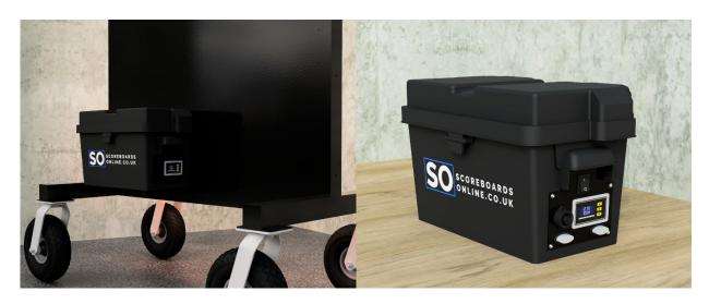
On the side of the battery box, underneath the power switch(es) you will see a small control panel. This is protecting the battery from being run too low which will cause irreparable damage to the battery itself. This works by monitoring the voltage remaining in the battery. When the battery is fully charged it will typically indicate 12.5 to 13v and show 100% capacity.
